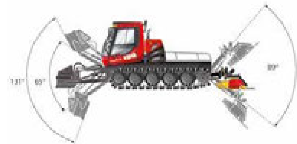
Extreme agility of the front and rear attachments for perfect shaping and reshaping.
