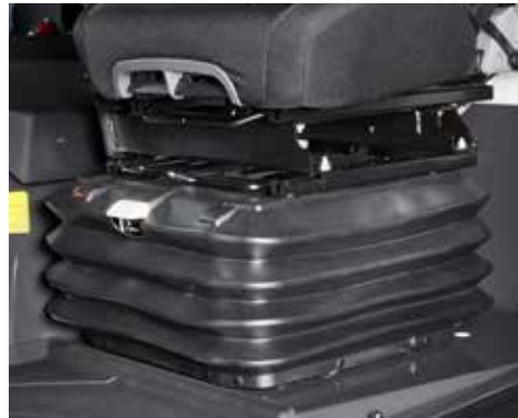
Driver's seat with air-sprung heavy-duty seat frame for healthier working and improved ride comfort.
