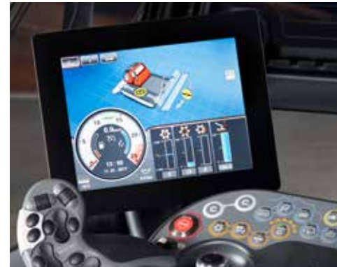
Patented iTerminal with optimized user guide thanks to color labelling of the active areas of the vehicle.
