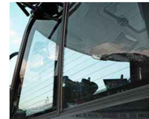
Dual sliding side windows, heated in any position, for optimum lateral visibility.
