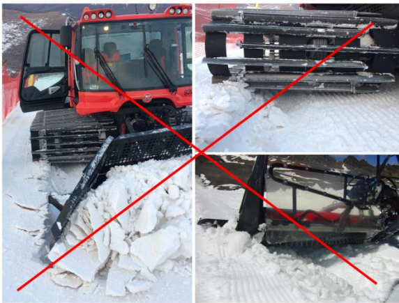
Incorrect opening angle
