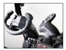
The joystick is for controlling the functions of the auxiliary equipment (blade and tiller), and also for controlling additional functions, if any.
