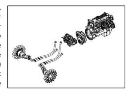
A hydrostatic drive is a propulsion system in which a liquid is pressurized in order to drive machinery and perform work. The term "hydrostatic" refers to the conversion of energy from flow and pressure. The biggest advantages of a hydrostatic drive system are continuous acceleration and wear-free deceleration of the vehicle.
