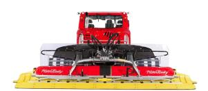
The **contact bar** consists of individual elements that are interconnected much like those of a windshield wiper system. The contact bar lies on the finisher and by exerting pressure it compacts the snow processed by the tiller shaft..
