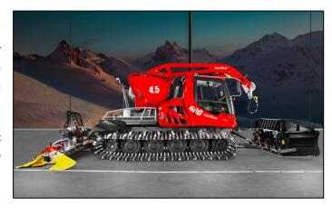
The winch body houses the winch drum with the winch cable, a reduction gear assembly with hydraulic motors and the cable reeling system. When switched off, the winch can be slewed through 360 ° by the operator. When in work mode, the winch slews freely on the slewing ring, so it is always facing in the direction of the winch cable.
